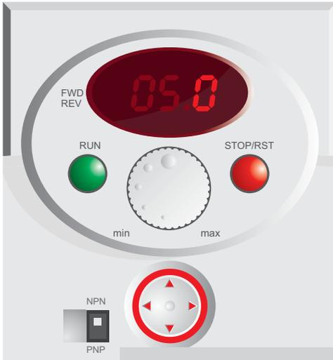
**6.4 Use the left and right arrows on the navigation pad to move between digits. Use the up and down arrows to increase or decrease the digit value.**
