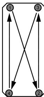
**Fig. 1-15:** Tightening sequence to mount the module to the heatsink
