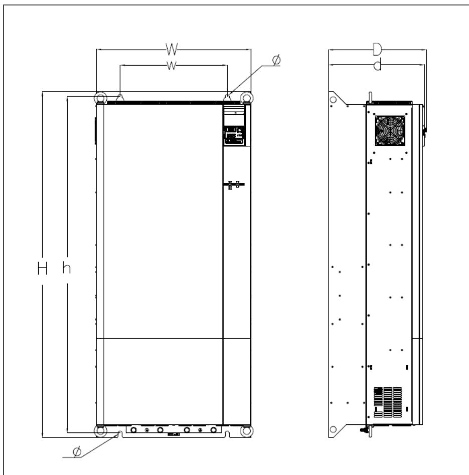
Fig. 1-11: EFC 5610 315K dimensions figure (3P 380 VAC)
