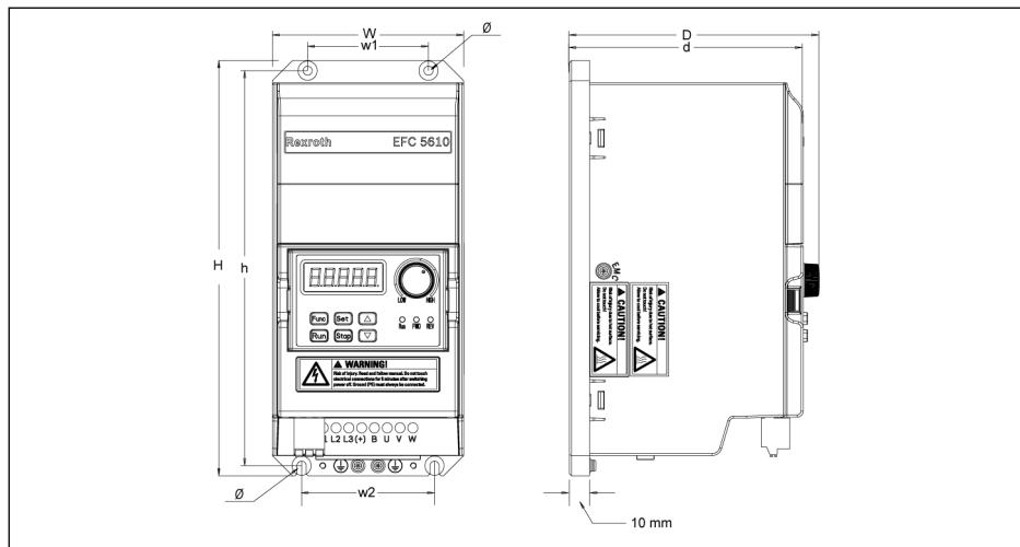
Fig. 1-12: EFC 5610 0K40...4K00 dimensions figure (cold plate, 1P 200 VAC / 3P 380 VAC)
