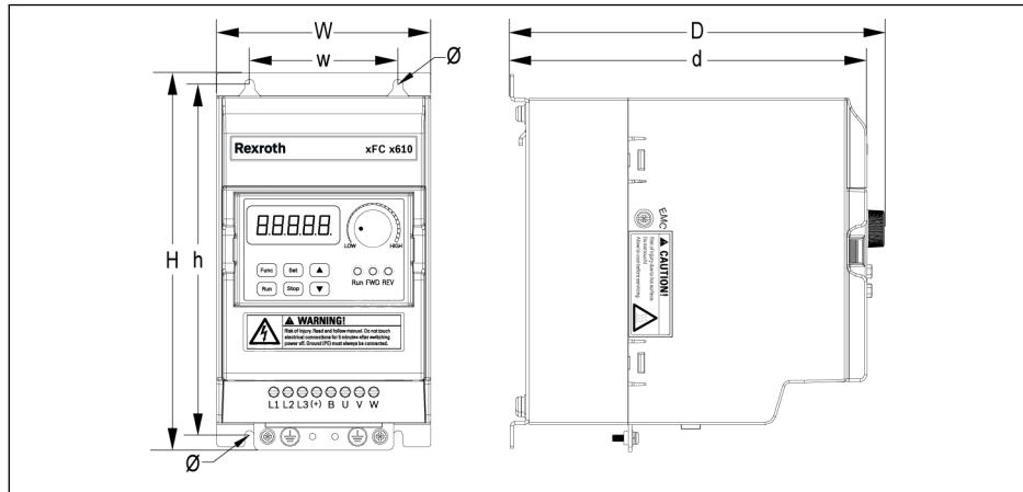
Fig. 1-1: EFC x610 0K40...4K00 dimensions figure (1P 200 VAC / 3P 380 VAC)
