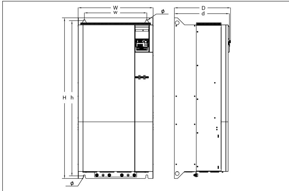
Fig. 1-10: EFC 5610 200K...250K dimensions figure (3P 380 VAC)
