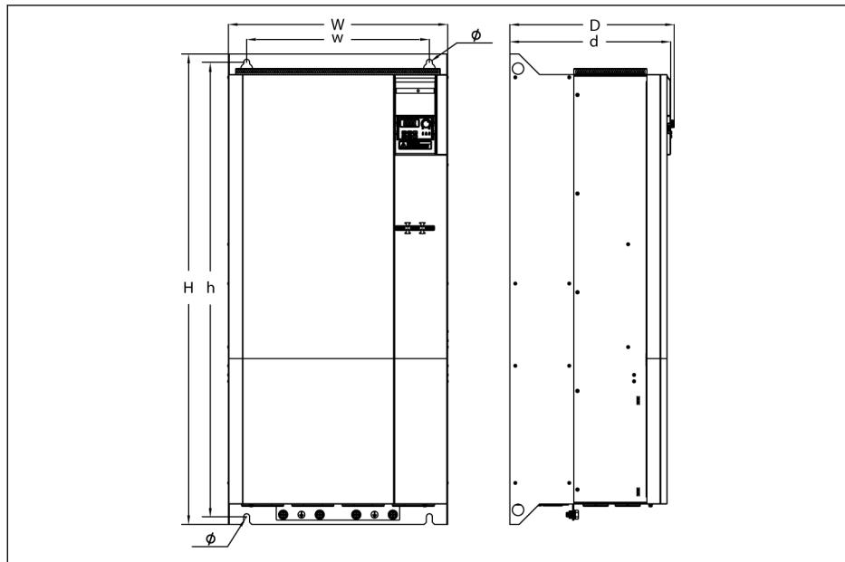
Fig. 1-9: EFC 5610 160K dimensions figure (3P 380 VAC)
