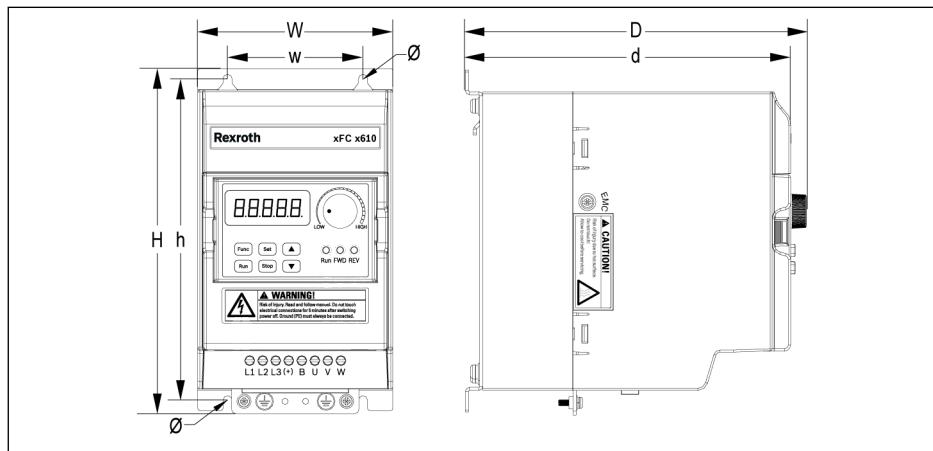
Fig. 1-2: EFC x610 0K40...2K20 dimensions figure (3P 200 VAC)
