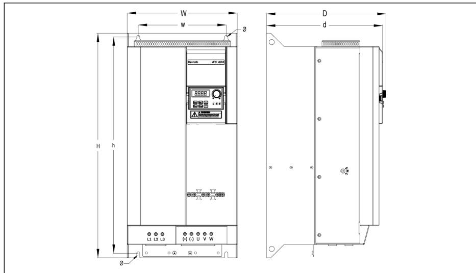
Fig. 1-5: EFC 5610 30K0...37K0 dimensions figure (3P 380 VAC)
