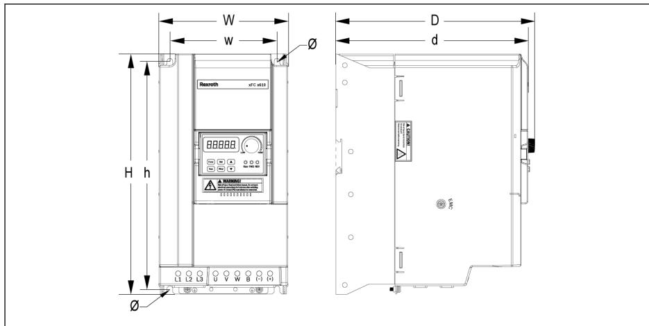
Fig. 1-3: EFC x610 3K00...11K0 dimensions figure (3P 200 VAC)
