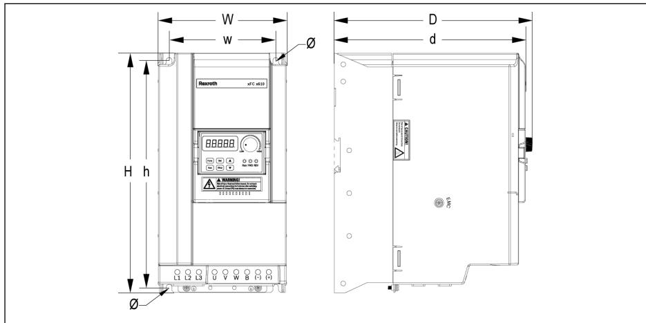
Fig. 1-4: EFC x610 5K50...22K0 dimensions figure (3P 380 VAC)
