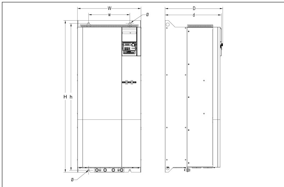
Fig. 1-8: EFC 5610 110K...132K dimensions figure (3P 380 VAC)
