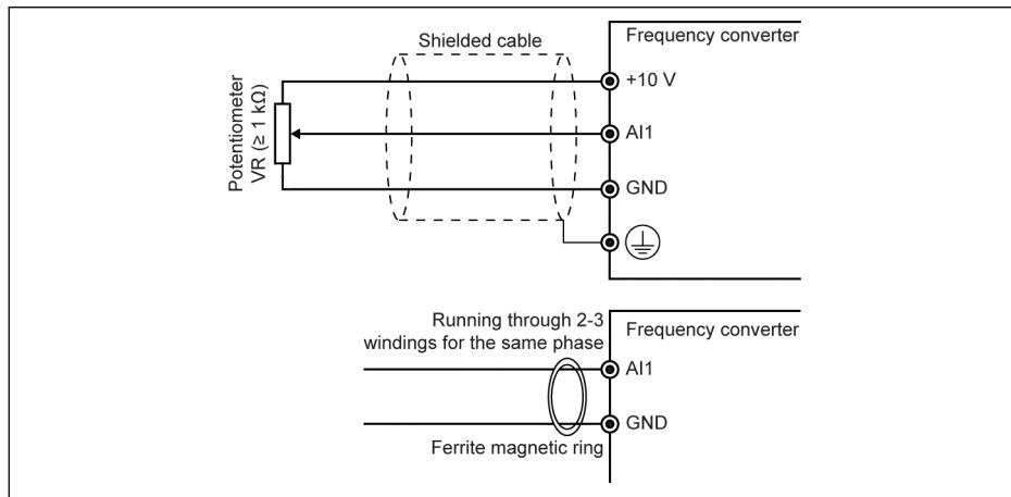
**Fig. 2-8:** Analog input terminals
