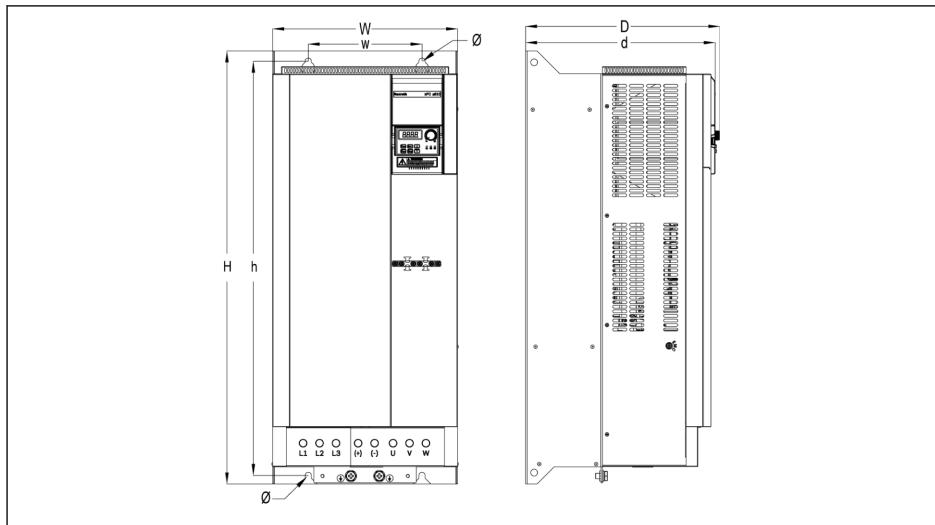
Fig. 1-7: EFC 5610 75K0...90K0 dimensions figure (3P 380 VAC)
